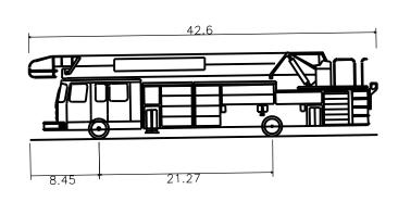
Pierce Quantum 105 Aer Truck Overall Length Overall Width Overall Body Height Min Body Ground Clearance Track Width Lock-to-lock time Wall to Wall Turning Radius
