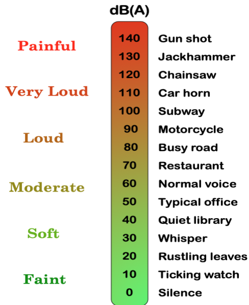
Figure 6: dB Values of Common Noise Sources, A-weighted
