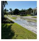
Summer water main breaks are often linked to our region's sandy soils and rainy season. Heavy rainfall can shift sand away from underground pipes, leaving them unsupported. At the same time, the added weight of saturated soil increases pressure on the pipes. Over time, this stress can create cracks that eventually lead to failures, as happened on Colonial Avenue.
