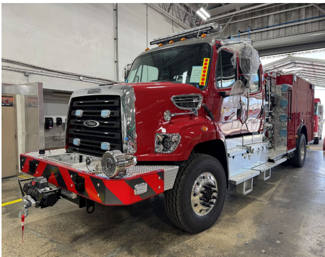
High Water Fire Engine under construction
