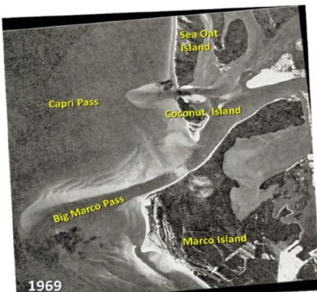
Natural inlet migration up-drift Up-drift erosion and downdrift sand spit growth (Dabeels and Moore 2014)
