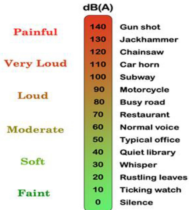
Figure 6: dB Values of Common Noise Sources, A-weighted
