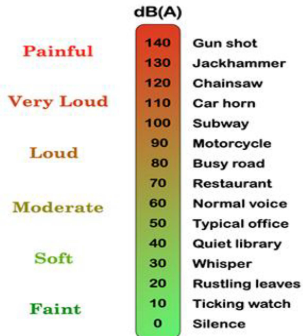
Figure 6: dB Values of Common Noise Sources, A-weighted
