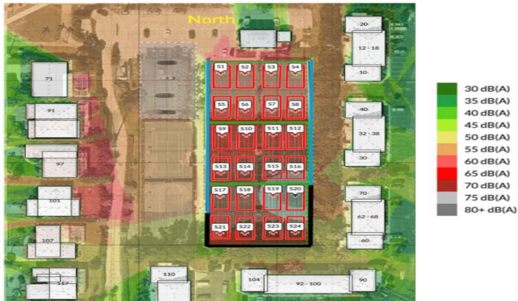
Figure 11: Noise Map. 12-Foot-High Barriers to the East, West and 16-Foot-High Walls to the South-West, South-East and South
