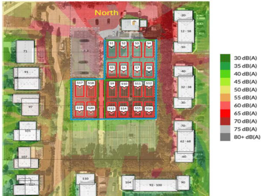
Figure 12: Noise Map, L-Shaped Expansion with 12-Foot-High Barriers to the East, West and South
